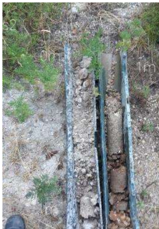
Figure 29 : Lithologie sondage S2
